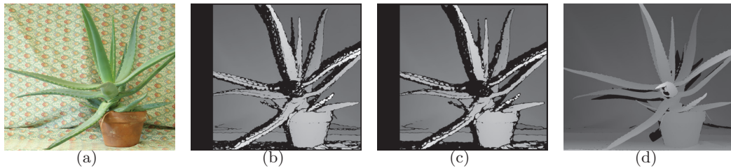
Figure 11: Increasing the window size for BM. (d) is the ground truth data to compare the disparity maps
