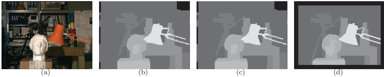
Figure 13: Resulting disparity maps for the Tsukuba image set created with the graph cut algorithm. (d) is the ground truth data to compare the disparity maps
