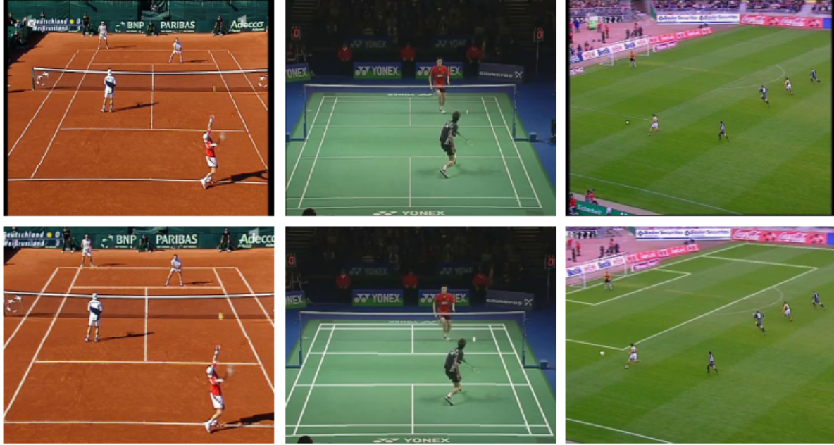
Figure 4. Examples of tennis, badminton, and soccer videos adapted to a resolution of 240x192 pixels. Top row: scaled. Bottom row: adapted with our advanced video retargeting approach ( \gamma = 3.0 ). Court lines in the background are much easier to see.
