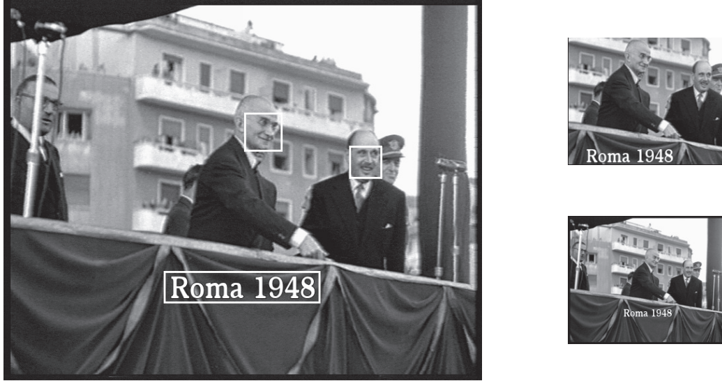
Figure 5. Sample frame with three automatically detected feature regions. Eight possible combinations of these regions are analyzed in order to find the maximum information value.
