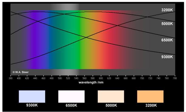
**Black-body radiation curves (vertical scale is linear):** If your computer and monitor adhere to the sRGB specification (your monitor color-point should be set to 'sRGB' or '6500K') then the sample colors should be colorimetrically-accurate.
