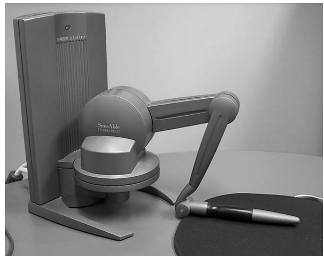
Figure 1. Sensable Phantom Haptic Pen.
