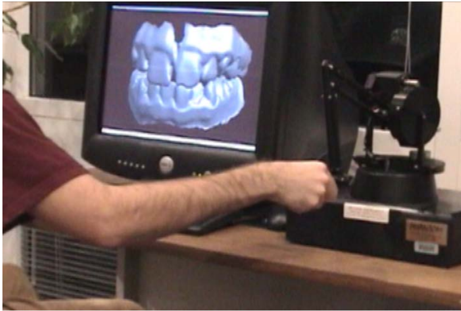
Figure 1: Example of Haptic Rendering. A person manipulates a virtual jaw using a haptic device (shown on the right of the image), and the interaction between jaws is displayed both visually and haptically.
