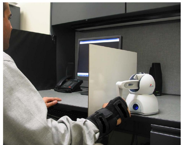
Fig. 1. The experimental setup: the PHANTOM TM haptic device and a subject.
