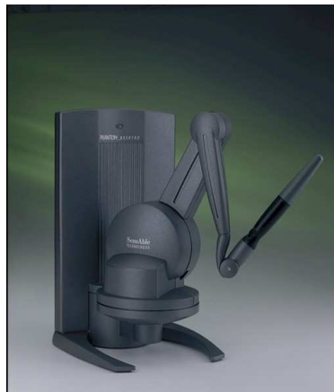
Figure 3: Sensable Phantom haptic device [3]
