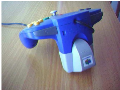
Figure 1: Evolution of haptic devices. Left: Nintendo Rumble Pak attached to video game controller (en.wikipedia.org). Right: Haptic Pen [7]
