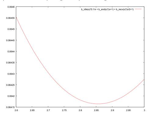
The optimal preamble for this scenario is at about 2.85 times a frame length.
