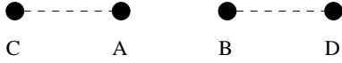
Fig. 2. Neighboring nodes A and B have different schedules. They synchronize with nodes C and D respectively.
