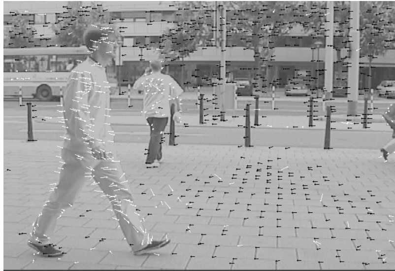
(a) Detected correspondences (outliers found by RANSAC are drawn in white color).
