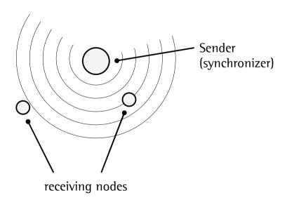
The signal propagation time is (almost) negligible. The source for variance in the measurement is the time different nodes need to receive the signal. All kinds of delays at the sender side do not play an important role since they are the same for every receiver.
