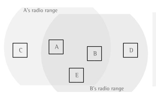
Remark: In reality, in addition to its transmitting range a sender also has a disturbance range, in which its packets aren't understood any more, but still cause collisions. The circular resp. spherical area around a sender is a simplification, too. By interaction with the environment the real reception areas look different in most cases.
