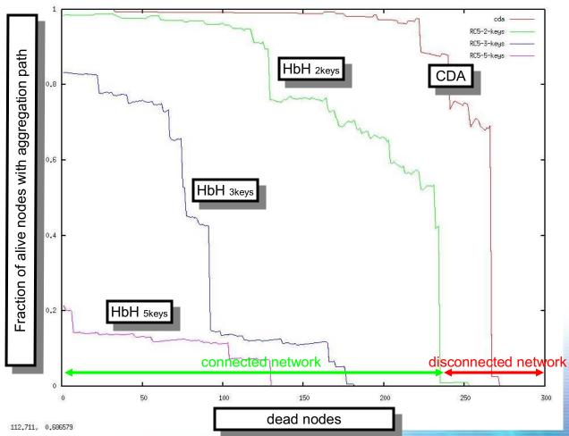
Glomosim: one RR with 318 nodes, static radio range, 20 neighbors, 10 min simulation time...
