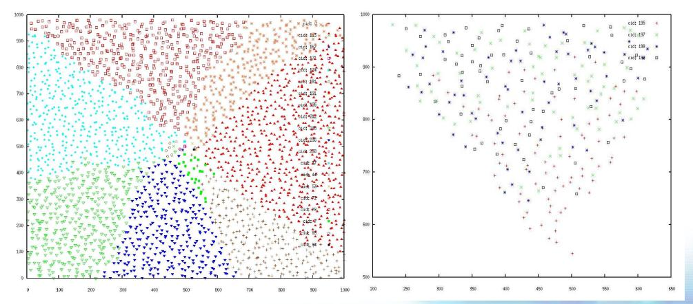
Glomosim: 2548 nodes 1000x1000, static radio range, 20 neighbors, 10 min simulation time...
