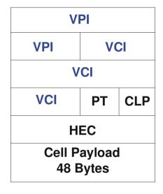
GFC: Generic Flow Control VPI: Virtual Path Identifier VCI: Virtual Circuit Identifier
