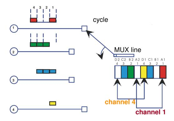
We observe: For **STM lines**, switching simply means a re-ordering of the time slots!
