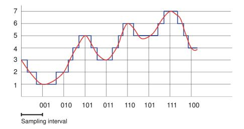
The combination of the steps sampling, quantization and binary coding is called **Pulse Code Modulation (PCM).**
