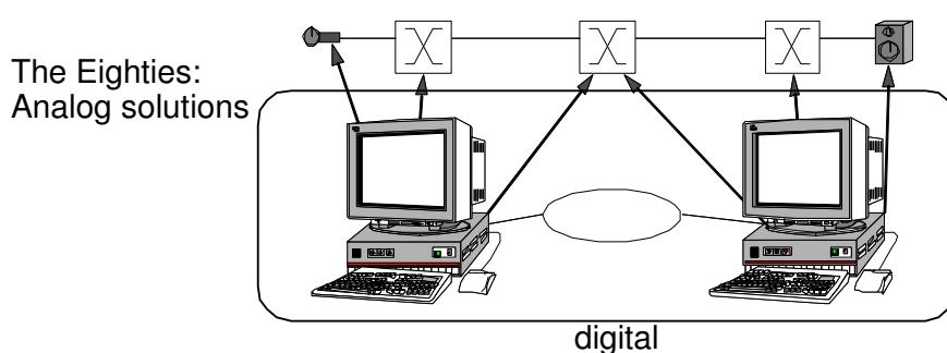
Computers control the analog media streams, e.g., via cross-connect switches.
