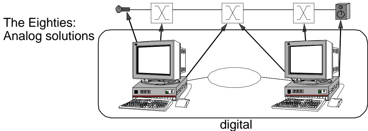
Computers control the analog media streams, e.g., via cross-connect switches.
