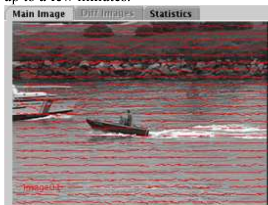
Fig. 36 The resulting motion vectors are displayed in the frame
