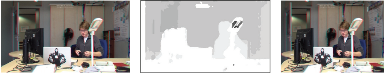
Figure 1: Example frame from the stereo sequence "office" that has been adapted by our new algorithm. The frames are shown in the anaglyph (red/cyan) format. Left: Original frame. Middle: Disparity map of the frame. Right: Result.
