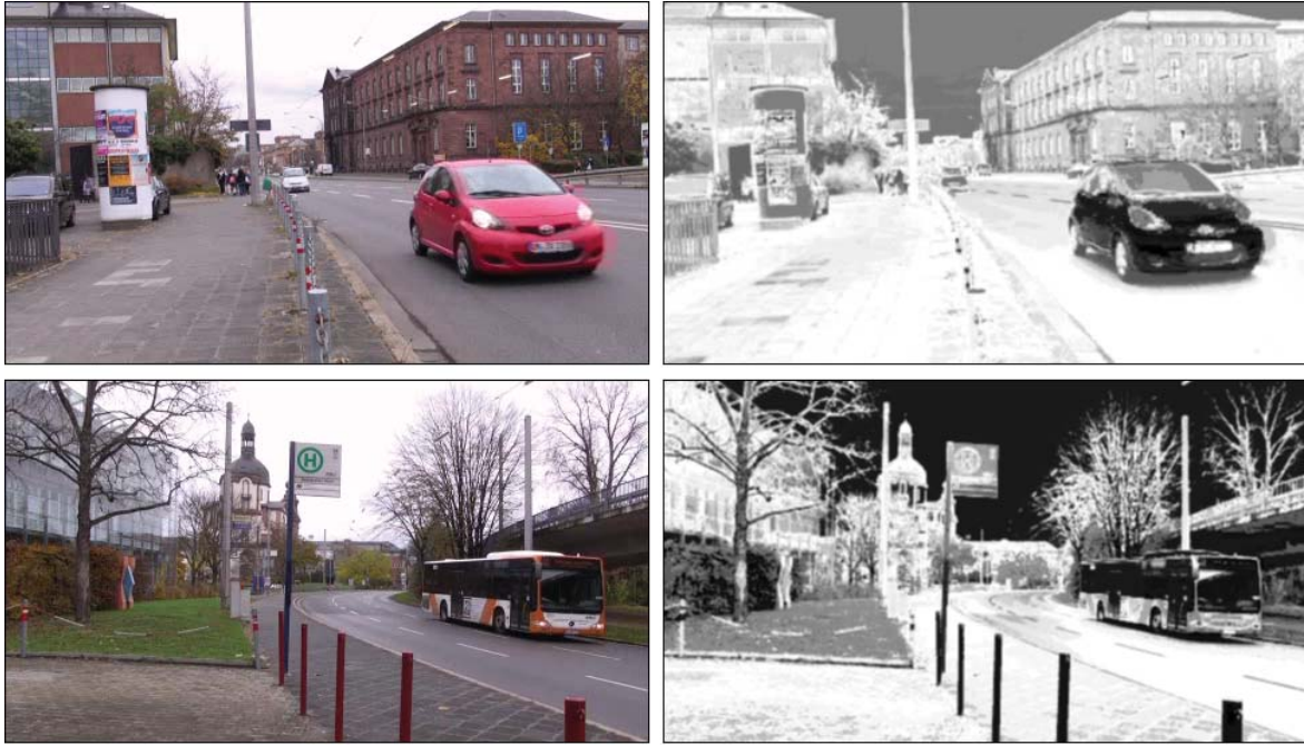
Figure 2: Left view of stereo videos and corresponding image saliency maps. Pixels with high saliency values are printed in dark colors.
