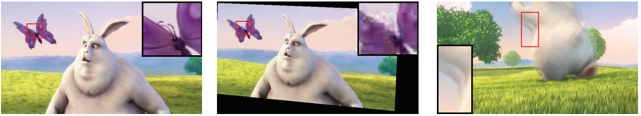
Figure 8: An original frame (a) after perspective distortion and compression with a very low bit rate (b). As in camcorderd copies, two successive source frames are blended into a copy frame in (c) (with a ratio of 50%).
