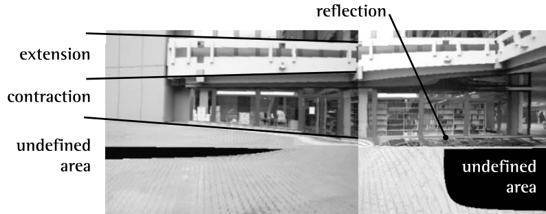
Fig. 8. The naive warping approach described in Section 3 creates four classes of artifacts, namely expansions, contractions, undefined areas, and reflections.
