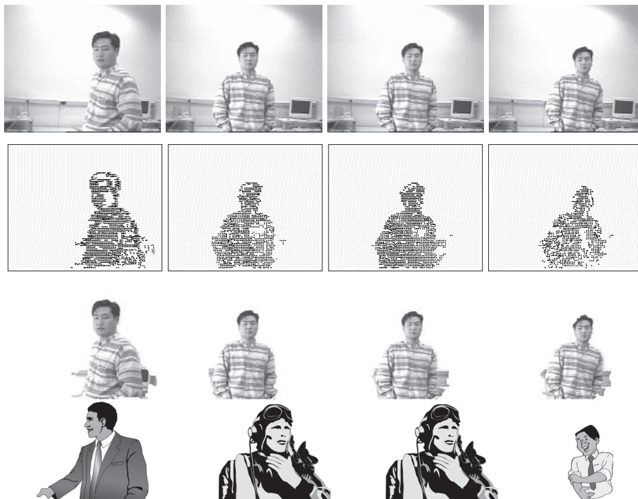
Figure 9: Segmentation and classification of the person sequence. Rows from top to bottom: (a) frames 25, 33, 34, 38, (b) motion estimation with hierarchical structure tensor, (c) tensor-driven active contour, (d) classification of the frames 25, 33, 34, 38, the top match is displayed.
