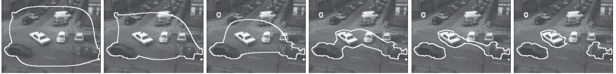
Figure 4: Tensor-driven geodesic active contour. From left to right: contour after 3000, 6000, 9000, 12000, 15000, 17392 iterations. Constant force c = 0.02 .
