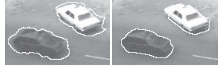
Figure 5: Contour refinement. Left: motion-based segmentation, right: motion-based segmentation with contour refinement (445 iterations, \tilde{C} = 1.5 ).
